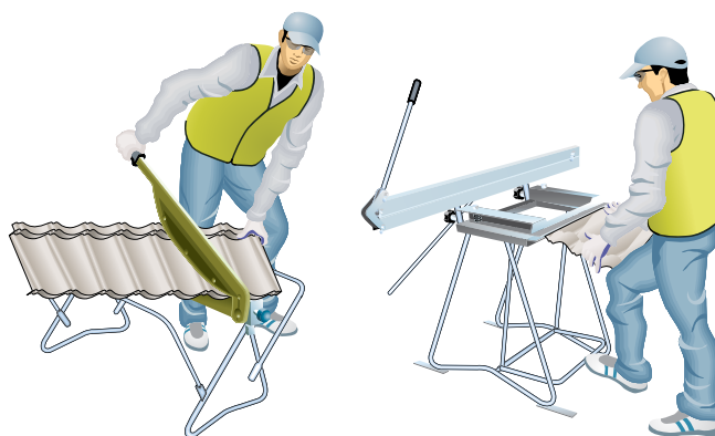
Figure 2.7.7.2 Valley tile being cut then bent
